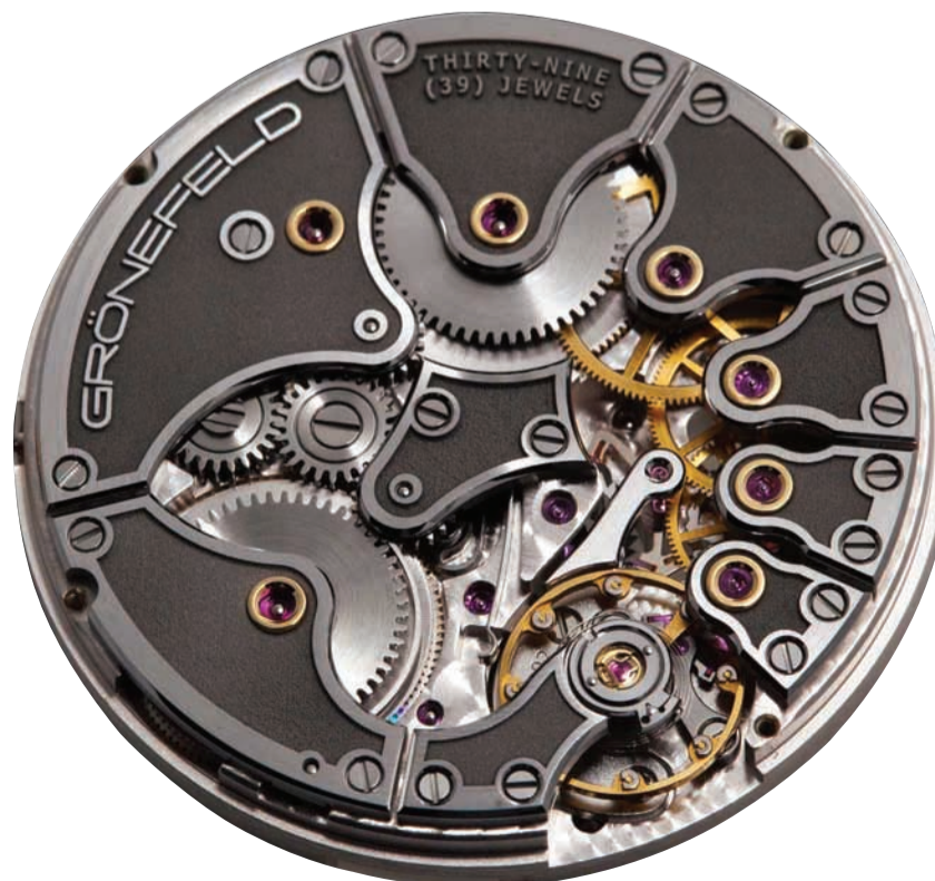
The Grönefeld One Hertz is both the world's first wristwatch with independent dead seconds, and is the only watch with all bridges made from stainless steel.
